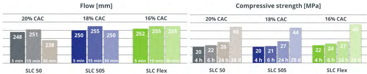
Fig. 3: Flowability [mm] after 5 min, 15 min, 30 min (left) and Compressive strength [MPa] after 4h, 6h, 24h, 28 d (right) of SLC 50, SLC 505 and SLCFlex
