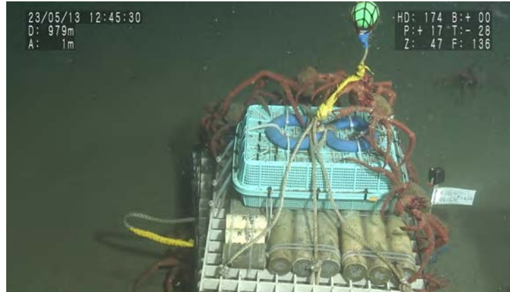
Figure 1. Deep-sea exposure site at 980 m depth showing specimen placement. Photographs courtesy of the Japan Agency for Marine–Earth Science and Technology.
