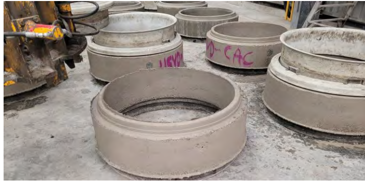
Figure 2. Precast access chambers manufactured using specialty binder concrete during pilot-scale casting trials.
